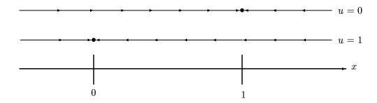
It is easily seen (cp. the figure) that (6.1) possesses an (invariant) control set C = [0, 1]. All solutions starting outside C can be steered to C but no trajectory can leave C.
