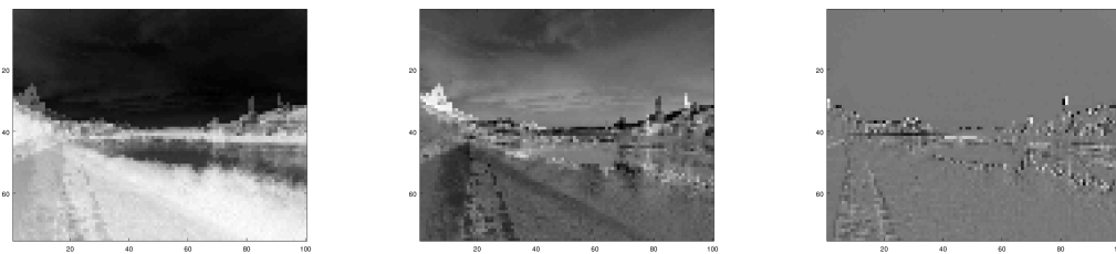
Figure 5.3: The singular vectors of the image matrix. The respective singular values are 2.1 \times 10^4 , 2.8 \times 10^3 and 1.2 \times 10^3 , hence the first image part dominates significantly.
