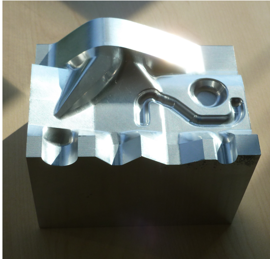
Figure 1.2: A CNC test workpiece for testing how well the geometric model is really generated physically.
