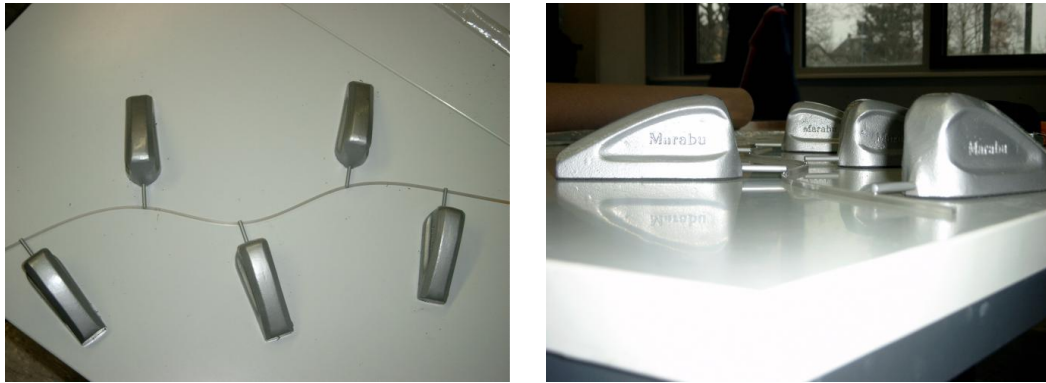
Figure 4.13: A real world spline, consisting of a bendable ruler and weights, called ducks that tie it to certain places where the curve has to interpolate. The spline was given to the Numeric Mathematics group of Giessen by H. Hollenhorst.
