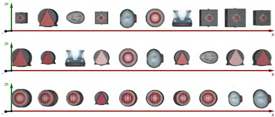
Figure 4.6: The graphic shows the first 10 shapes of the three chosen single transformation test queries, which should be comparable easy but returned quite bad results for both models. The chosen queries are 1: Cuboid/Rhomboid presented in row one, 2: Prism/Cylinder in row two, and 7: Cylinder/Ellipsoid in row two.
