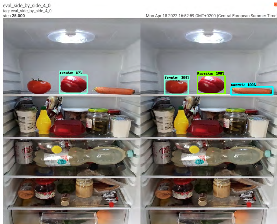
Figure 5.3.4: The model could not detect the carrot and the tomato and falsely predicted the red pepper
