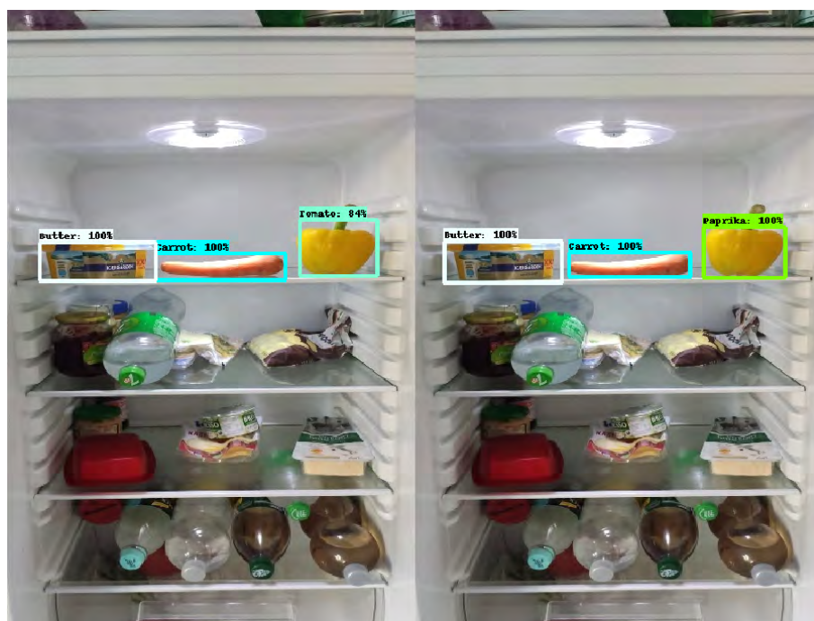
Figure 5.4.4: The result shows the model detecting the pepper as a tomato and correctly detecting the other classes
