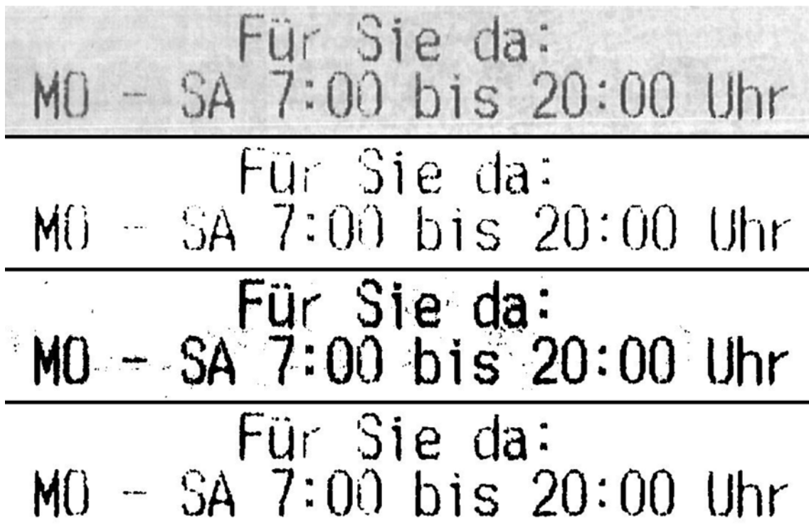
Figure 5.6: A piece of a receipt in grayscale (top), binarized with a threshold of 127 (center-top), 200 (center-bottom) and 161 (bottom). The threshold of 161 has been calculated by using Otsu's method.
