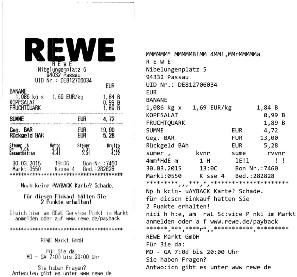
Figure 5.23: A binarized receipt image and the text recognized by OCRAM .
