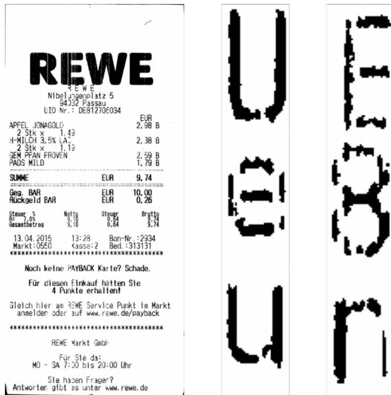
Figure 3.2: A receipt with white vertical flow marks (visible on the top logo) and characters extracted from this receipt
