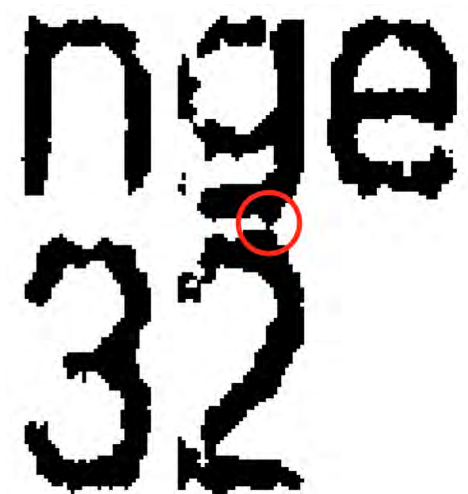
Figure 5.9: The “g” and the “2” are connected via one black pixel. This results in both lines being detected as one when using the white row strategy.
