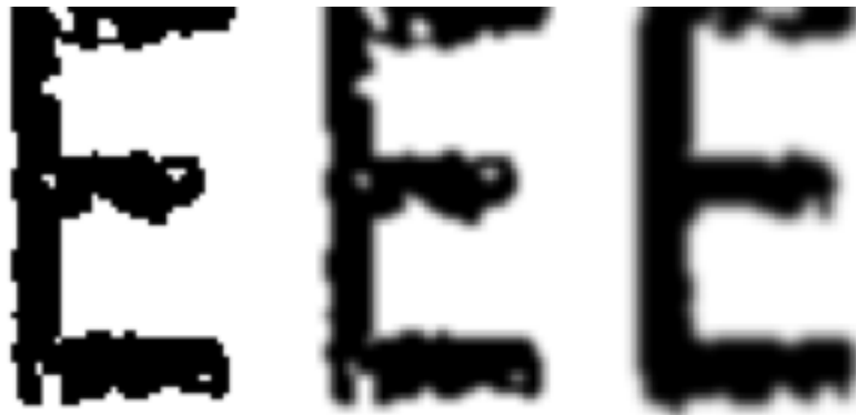
Figure 5.21: A character image (left) and the image after applying a binomial mean filter with radius 1 (middle) and radius 2 (right).
