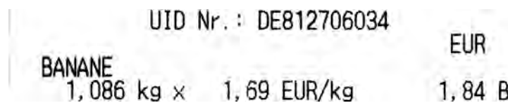
Figure 5.10: The line “EUR” has less black pixels per row than the other lines. This can cause problems for an inaccurate threshold in relative pixel count strategy.
