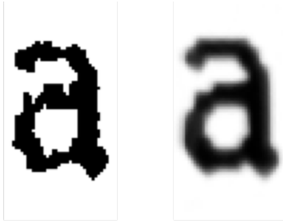
Figure 2.3: A single extracted character and the associated template image (see section 5.4.2 for details). The extracted character is the first occurrence of an lowercase “a” in the receipt from figure 2.2 (in “Nibelungenplatz”)
