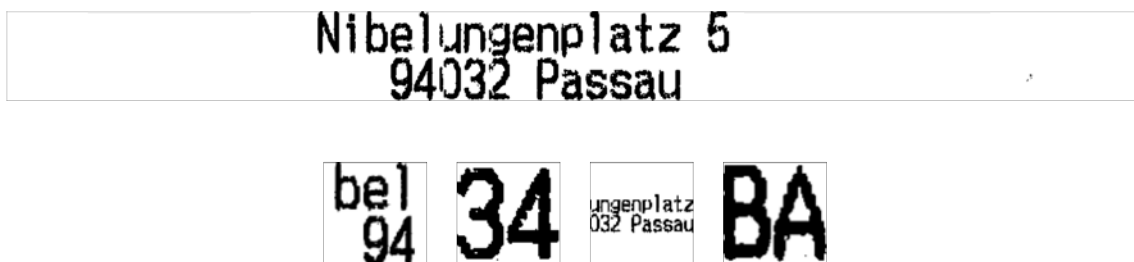
Figure 5.1: Top: Two lines are segmented as one by Java OCR . Bottom: Four characters, as they have been segmented by Java OCR .
