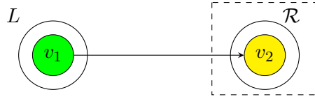
Figure 4.11: An SCC L = \{v_1\} and SCC \{v_2\} \in \mathcal{R} with vertex set X' = \{v_2\} highlighted in yellow and P = \{v_1\} highlighted in green.
