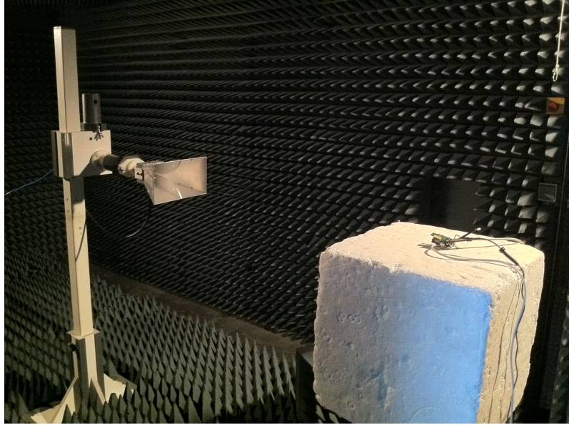
Figure 17. Absorber hall with jamming device and clusterhead.
