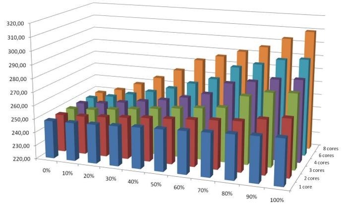
Fig. 2. Power consumption of a G-Lab server with different loads on the cores of its CPU
