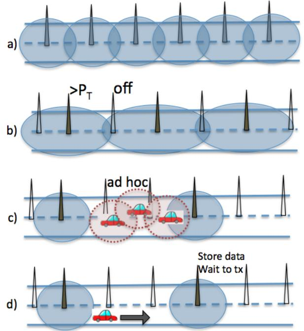
Fig. 3. Use case: the vehicular scenario. All BSs are on (a), EE with increase transmission power (b), EE with ad hoc networking (c), EE with DTN approach (d).
